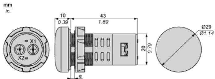
e : Clamping thickness: 1 to 6 mm/0.04 to 0.24 in.
